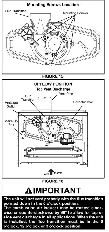
If necessary, reposition the combustion air inducer, pressure switch and/or make-up box as needed per the following steps. See figures 17 through 21.
